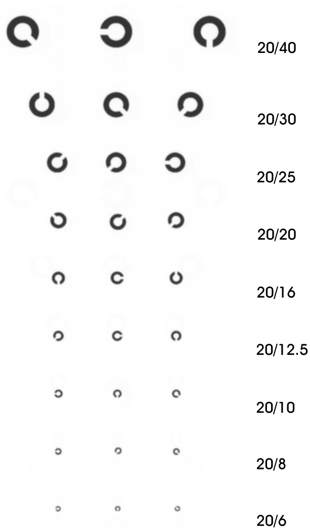
Fig. 2.20. Vision Chart for a 20/10 eye (with Styles-Crawford effect) corrected with a segmented active mirror. The mirror parameters were mirrorsize 37\ \mu\text{m} , width of the arms 3\ \mu\text{m} , noise in the stroke amplitude 30 nm and a PV of also 30 nm per submirror
