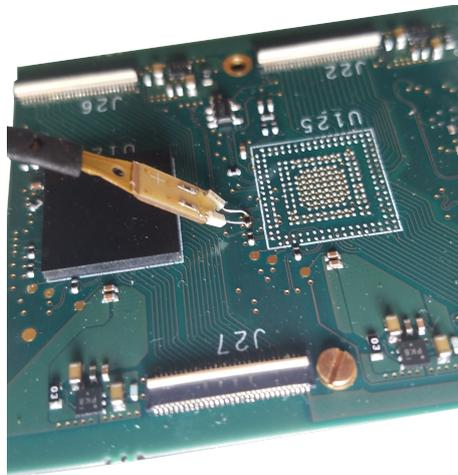
Figure 11: **D13000PS probe soldered to a reset termination resistor.** The resistor next to the soldered one terminates the CLK line. As this photo represents an early measurement setup, the TMB was not equipped with a all MuTRiGs.
