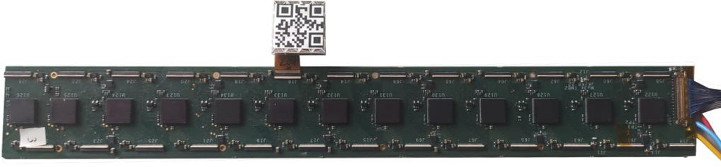
Figure 6: **TMB with one connected sensor matrix.** To the right, the DC voltage inputs (in colors blue, red and yellow), as well as the micro-coax are visible. The matrices can be connected to both long sides of the board and are mounted on the other side, while the flexprint is bent around the corners. [14]
