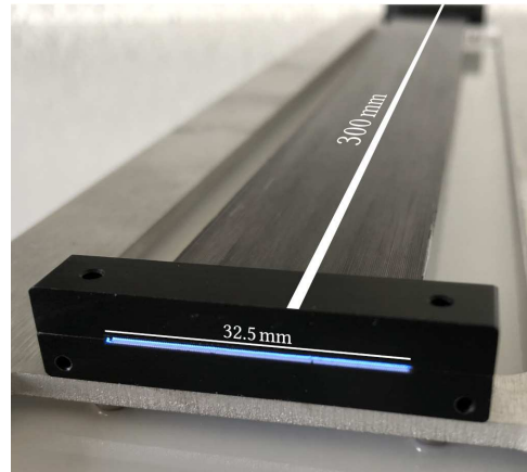
(b) Full size prototype of a SciFi ribbon.
